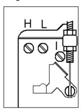
• Turn the idle speed adjusting screw (I) counter-clockwise until the drilling spindle stops rotating - then turn the screw approximately one half turn in the same direction.
